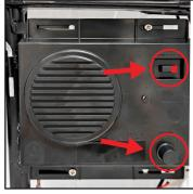
28. Turn the switch to the ON position to activate the item. Move in front of the item or make a loud sound (clap) to activate. Turn item OFF when not in use. Adjust volume control as needed.
