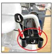
18. Insert the two metal posts on the LEFT ARM WITH HAND into the HEAD & TORSO FRAME WITH MODULE & CONTROL BOX. (MATCH J TO J)
